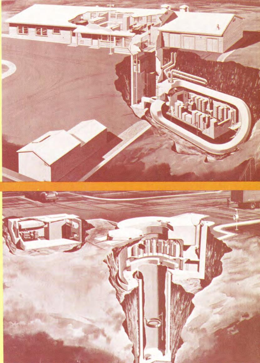
*These cutaway views, reproduced through the courtesy of AVIATION WEEK and Space Technology Magazine, show the details of a Minuteman site. Johnson controls are centered in the environmental control room at left of the silo proper, bottom view.*
