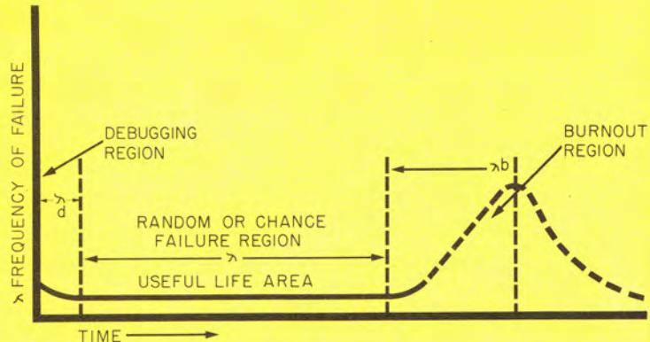
The "bathtub curve" is the nickname for the graph of a typical reliability formula. It shows the expected useful life of a part, such as a valve or thermostat, sandwiched between curves representing the production period or birth of the part, and its projected breakdown or old age.
